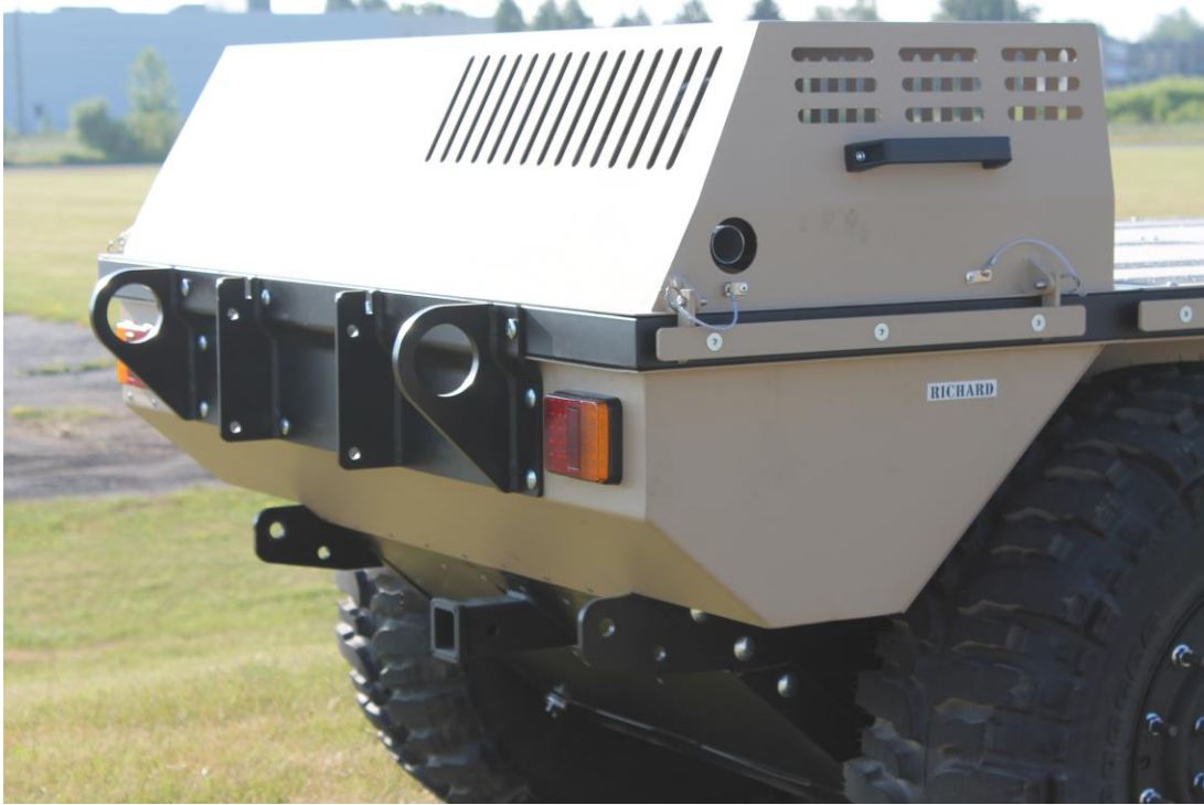
INTEGRATED REAR MOUNT DIESEL GENERATOR PROVIDES 13 kW OF ELECTRICAL POWER
